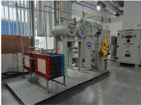
Process diagram and image of PEM based ECMR developed at ARCI with a hydrogen production capacity of 5.0 kg/day
