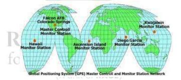
• There are ground stations which measures the signals from satellite and process the tracking data for computation of satellite co-ordinates and satellite clock parameter.
